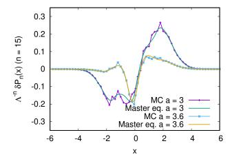
FIG. 6. Shape of the rescaled deviation  $\delta P_n(x)$  vs x from the equilibrium distribution at finite times (here n=15). The symbols show results of direct Monte Carlo and the lines show the results of the iteration of the Master equation; both methods are in good agreement. Same confinement and jump distribution as in Fig. 5.
